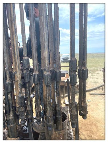
We poured 5 gallons of **ChainBreaker** super concentrate down the tubing so the microbes would *eat* the paraffin from the rods and break them free. After only 8 days the well was freed. The paraffin was sufficiently *eaten* to allow the rods and pump to be pulled up.
