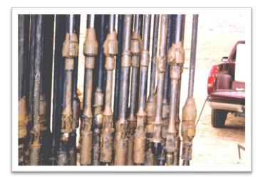
This picture is of rods which had been paraffined up and stuck in a 9,000 foot well in the Scott Field of Wyoming. A treatment of microbes was pored down the tubing and after two weeks operators were able to pull the rods. Note that almost all the paraffin was removed by the microbes during that time.
