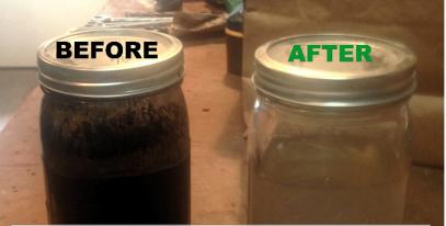
Water output from production separator **BEFORE** use of microbes. Contains 2% oil and iron sulfides Oil is now going into the going into the waterflood injection pump.
